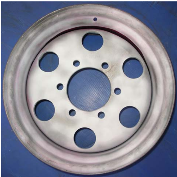
After 1 500 000 cycles radial fatigue no failure evident
