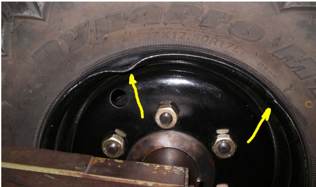
5 516 cycles - outboard flange crumpled (2 places) and lost all air
